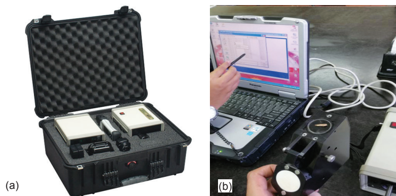
Figure 1. Instrument used in this study (a) a complete set of spectroradiometer, GER 1500 and (b) Spectral reflectance measurement for live and dead bagworms using calibrated probe; only one bagworm positioned on the probe during spectral measurement.
