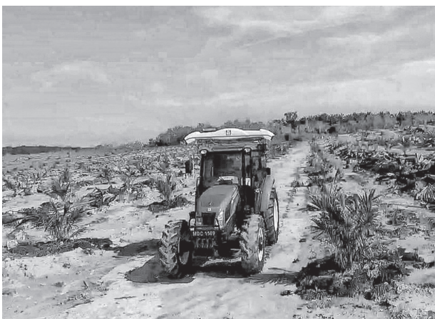
Figure 2. Autopilot tractor-mounted N-sensor is assessing N status on the immature palms in the study area.
