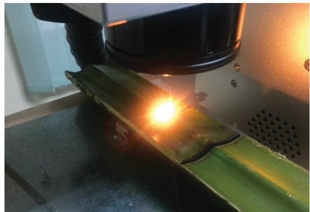
Figure 8. Laser cutting process of oil palm frond in laboratory condition.
