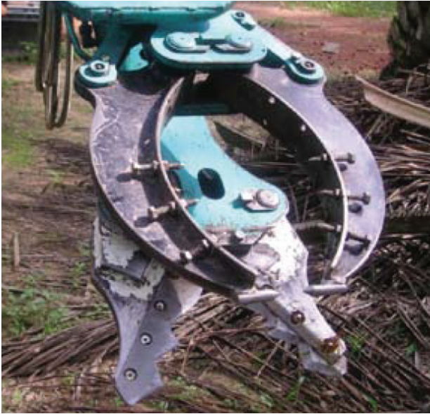
Figure 6. Oil palm FFB harvesting machine with grapple and scissor cutting mechanism.
