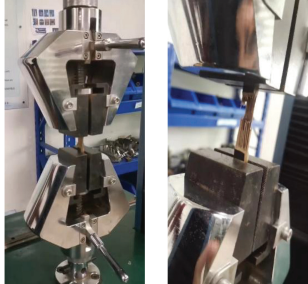
Figure 4. The measurement test of rupture modulus.
