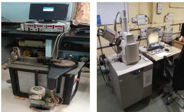
Figure 5. Experimental setup of the POD wear tester and SEM used in the study.
