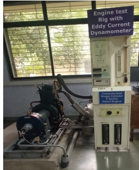
Figure 6. Experimental setup of the engine test rig.
