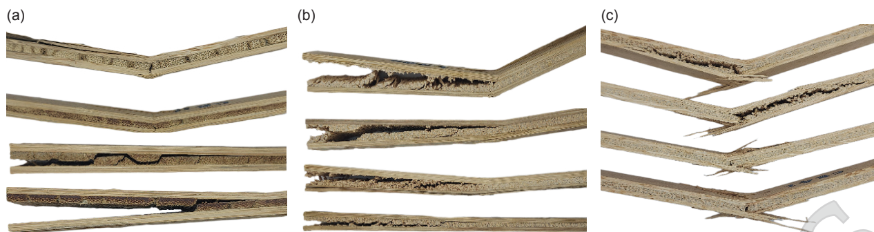
Figure 7. The failure mode of the test specimens after the bending test. (a) Bamboo mat panels, (b) hybrid panels and (c) OPT veneer panels.
