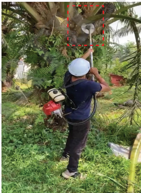
Figure 5. The cutting profile of oil palm fronds using circular blade cutter.
