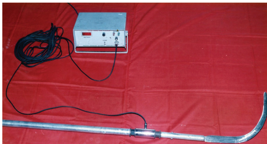
Figure 3. A view of the load cell and indicator connected between the pole and the knife.
