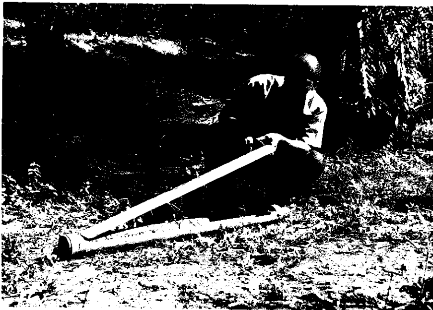
Figure 5. The soil column cylinder opened into two halves to reveal its soil sample intact.
