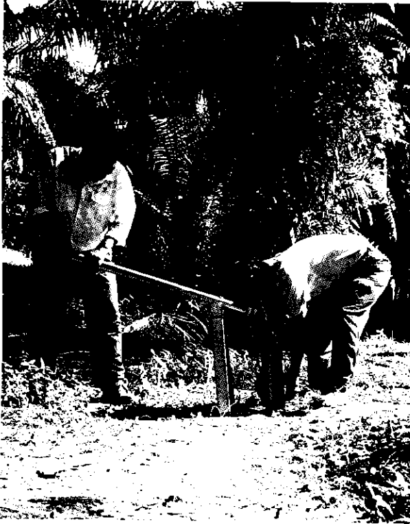
Figures 3 and 4. Pulling the soil column cylinder out with the lifting jack. A length of 2.5cm diameter steel chain was tied to the cylinder and attached to the lifting lever of the jack.
