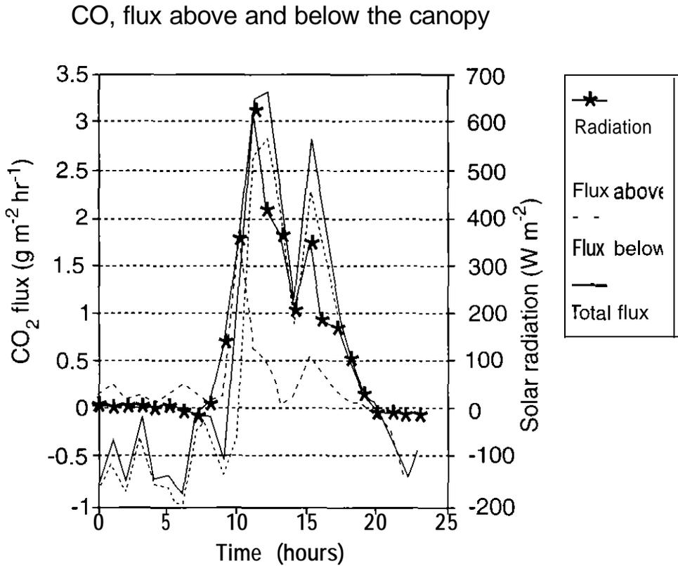
Figure 3. Hourly changes in below-canopy, above-canopy and total CO<sub>2</sub> flux in relation to above-canopy incident solar radiation, 21 December, 1994.
