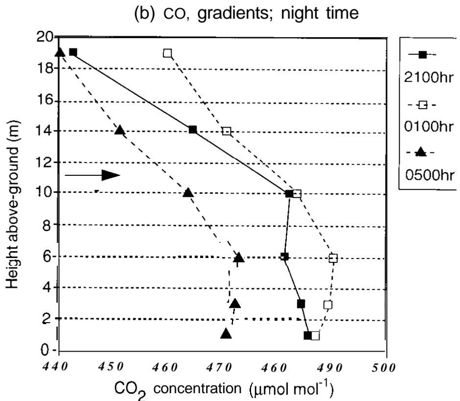
Figure 2. Examples of vertical gradients in CO<sub>2</sub> concentration within and above the canopy at different times; (a) during daylight and (b) during the night. Note difference in horizontal scales between (a) and (b). Arrows indicate top of canopy.
