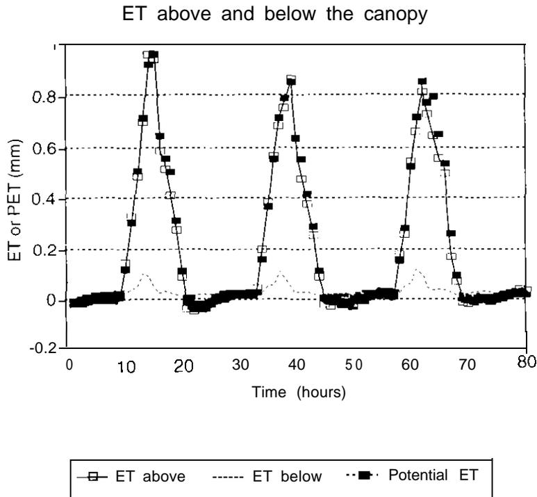
Figure 4. Hourly changes in total (above-canopy) and below-canopy evapotranspiration in relation to potential ET, 23 to 25 December, 1994.
