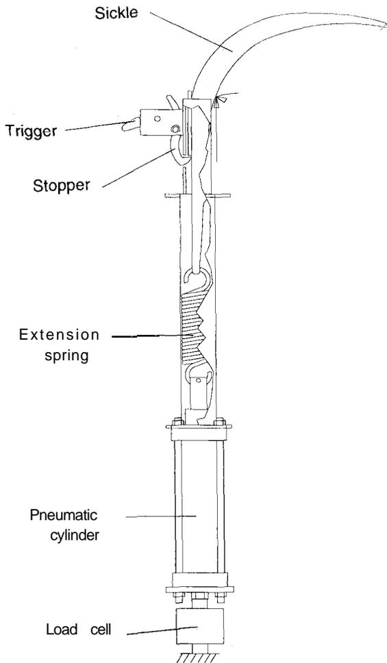
Figure 3. Experimental set-up to measure the reaction cutting force.
