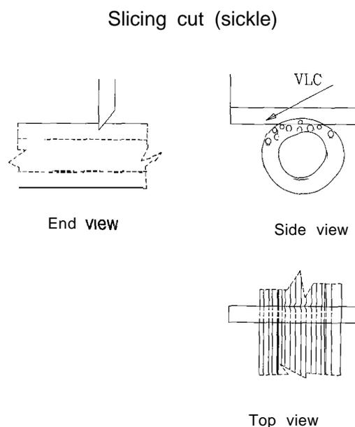
Figure 1. Views of slicing cut showing the directions of motion.
