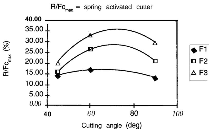
Figure 7. Effect of cutting angle on  $R/Fc_{max}$
