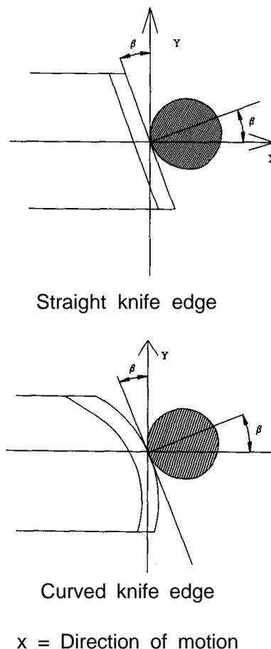
Figure 2. Oblique angle of straight and curved edges.
