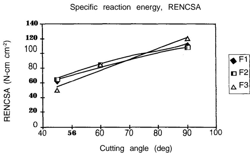
Figure 6. Effect of cutting angle on RENCSA.
