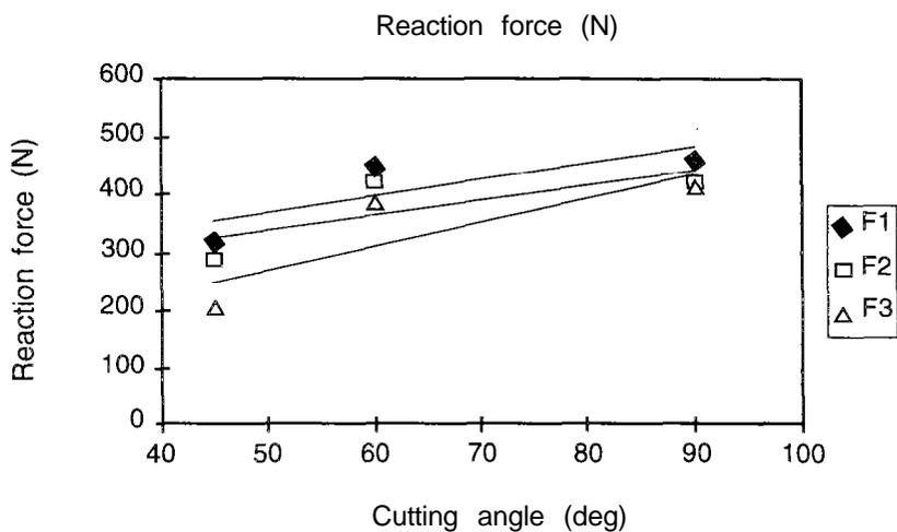
Figure 4. Effect of cutting angle on reaction force.
