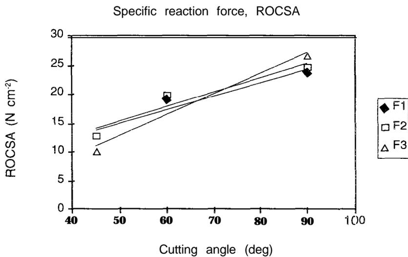
Figure 5. Effect of cutting angle on ROCSA.
