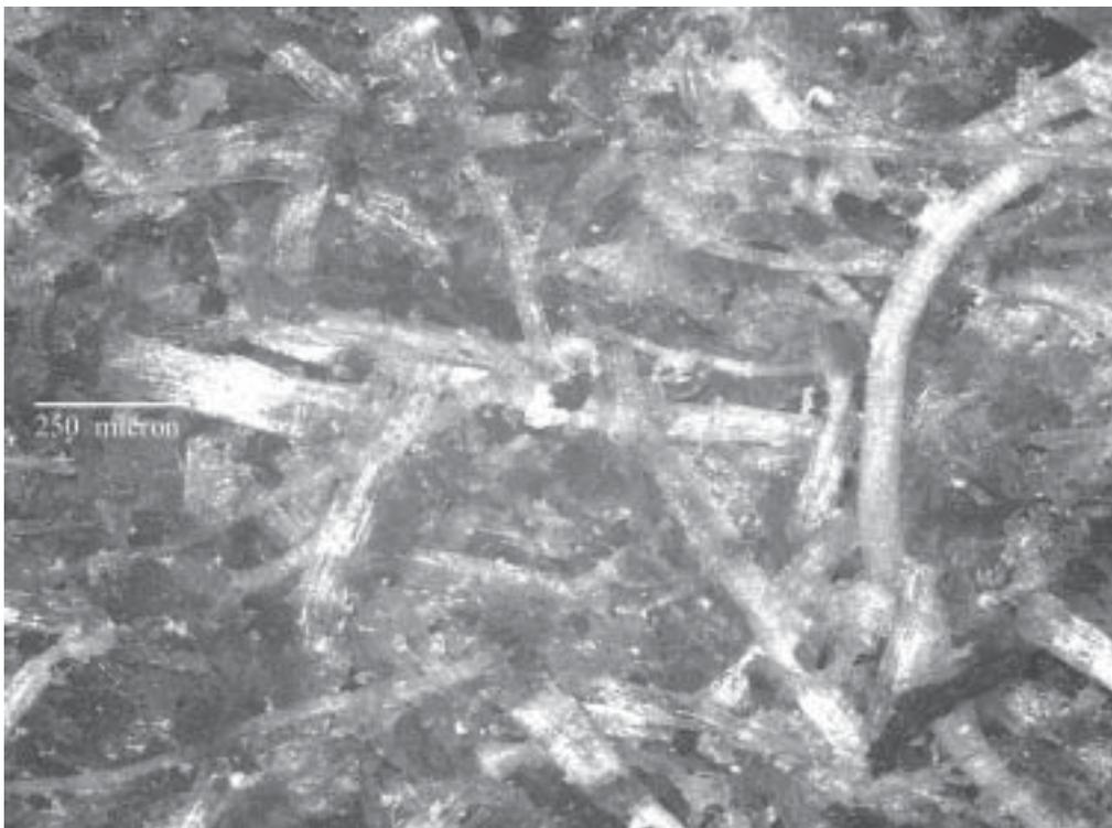
*Figure 4. Optical micrograph on the surface of biocomposite with blending ratio of 30:70.*
