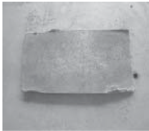
Figure 14a. Inlet chute liner before and after 200 operating hours.
