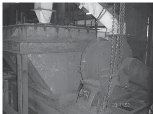
Figure 4. Rolek for multiple sizes of palm nut installed in Mills B and C.
