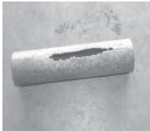
Figure 14c. Wearing carbon sleeves after 700 operating hours.
