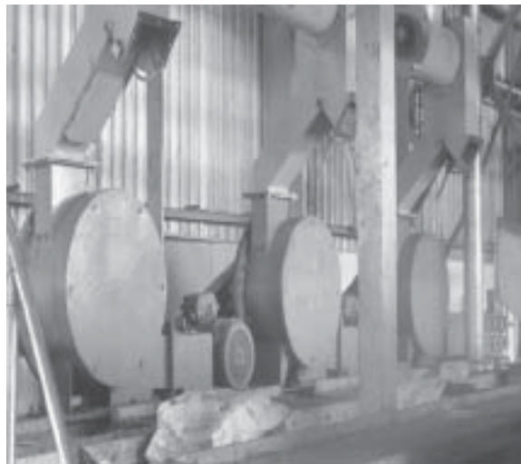
Figure 3. Three units of Rolek nut cracker for three different sizes installed at Mill A.
