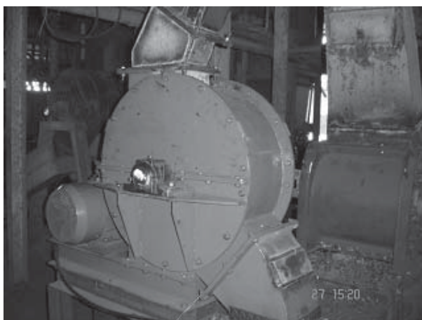
Figure 4. Rolek for multiple sizes of palm nut installed in Mills B and C.
