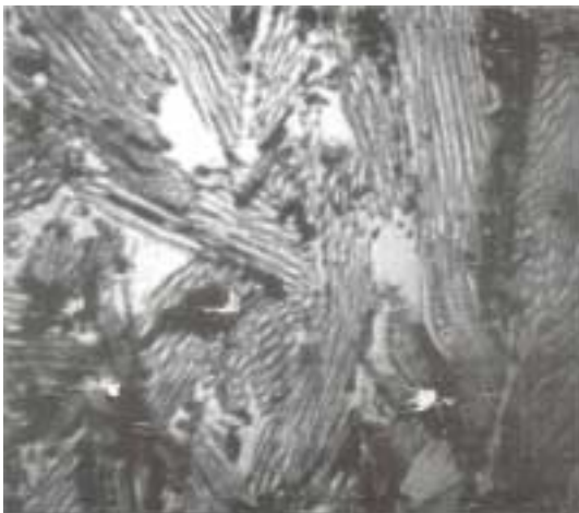
Figure 6a. Image of an empty fruit bunch laboratory panel along the z-direction (transverse section perpendicular to the height).
