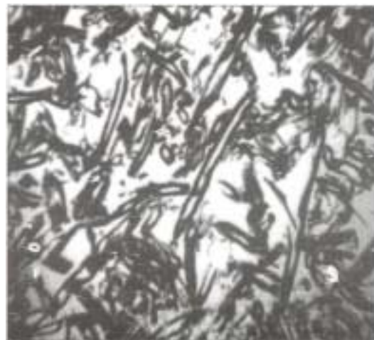
Figure 6b. Image of commercial medium density fibreboard panel along the z-direction (transverse section perpendicular to the height).
