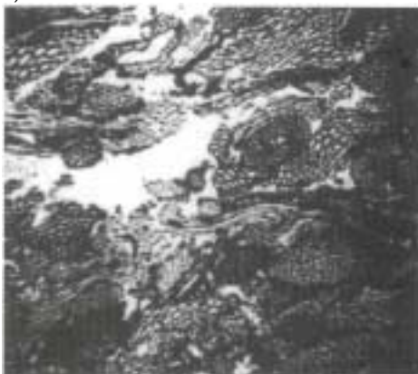
Figure 7b. Image of an empty fruit bunch laboratory panel along the y -direction (transverse section perpendicular to the length).
