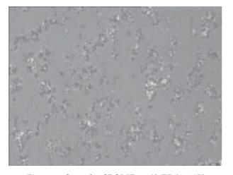
Figure 5. Crystals of POME + 5% EP (at 20X magnification).
