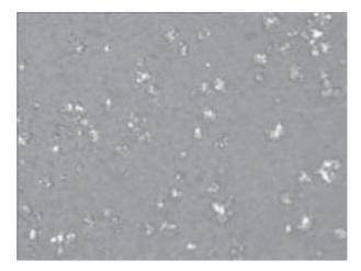
*Figure 4. Crystals of POME + 3% EP (at 20X magnification).*
