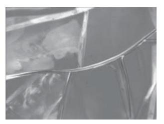
Figure 1. Crystals of POME without EP (at 20X magnification).
