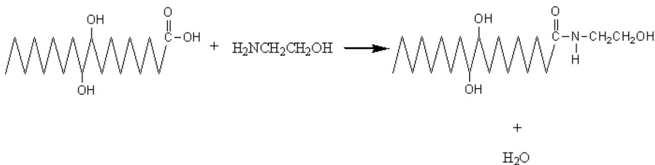
Figure 1. Reaction scheme of DHSA and ethanolamide.
