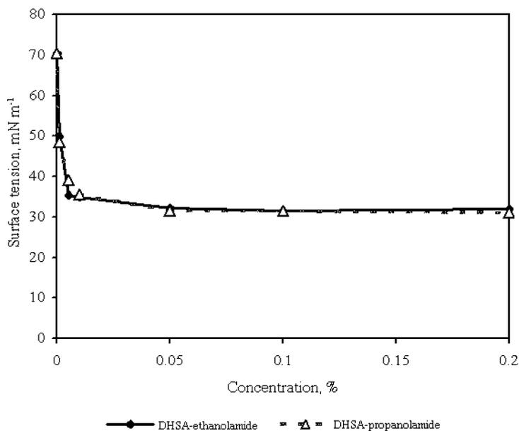
Figure 6. Surface tension vs. concentration of DHSA-alkanalamides.
