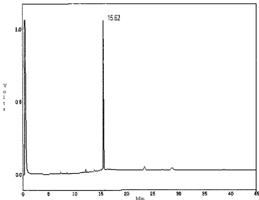
Figure 3. GC chromatogram of purified DHSA-ethanolamide.
