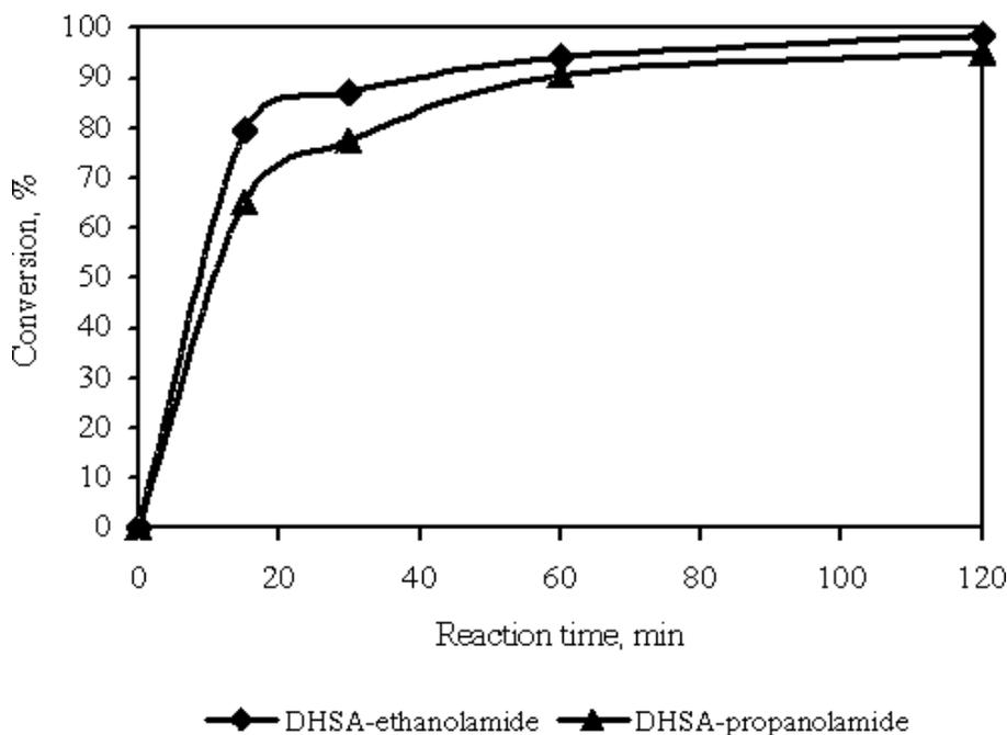
Figure 2. Effect of reaction time on amidation between DHSA and alkanolamines.
