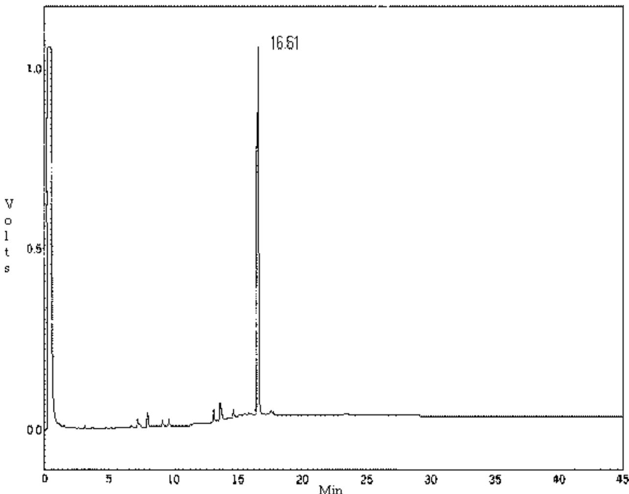
Figure 4. GC chromatogram of purified DHSA-propanolamide.
