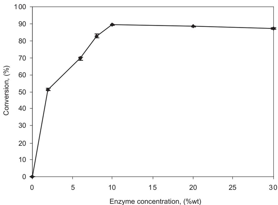
Figure 2. Effect of enzyme concentration on the esterification of DHSA and 1-octanol. Reaction conditions: reaction time, 3 hr; temperature, 50°C; agitation speed, 300 rpm.
