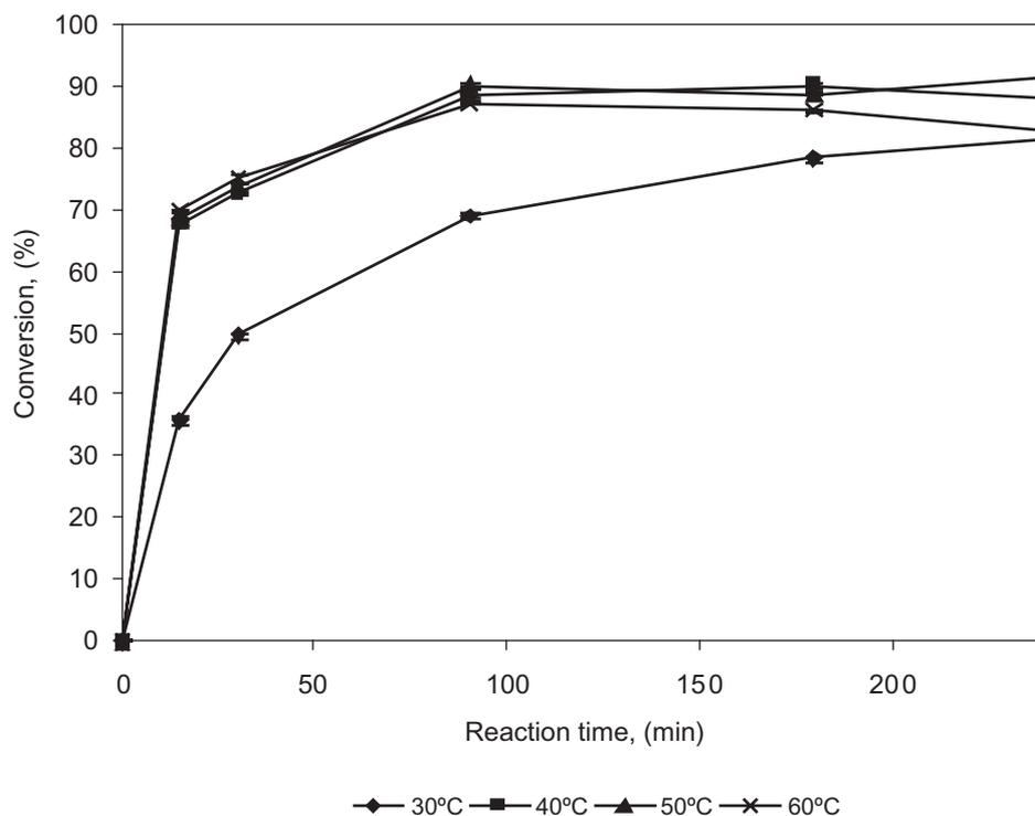
Figure 1. Time course of formation of octyl-9,10-dihydroxystearate by esterification of DHSA and 1-octanol at various reaction temperatures. Reaction conditions: enzyme concentration, 15% (w/w); agitation speed, 300 rpm.
