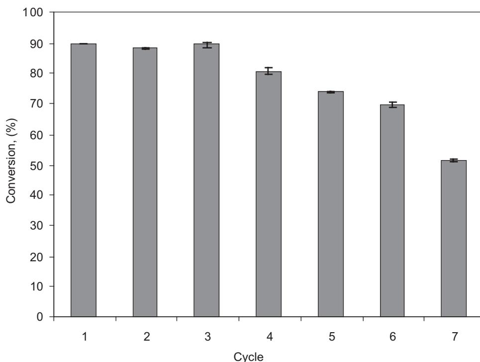
Figure 4. Reusability test for the immobilized enzyme in the esterification reaction system.
