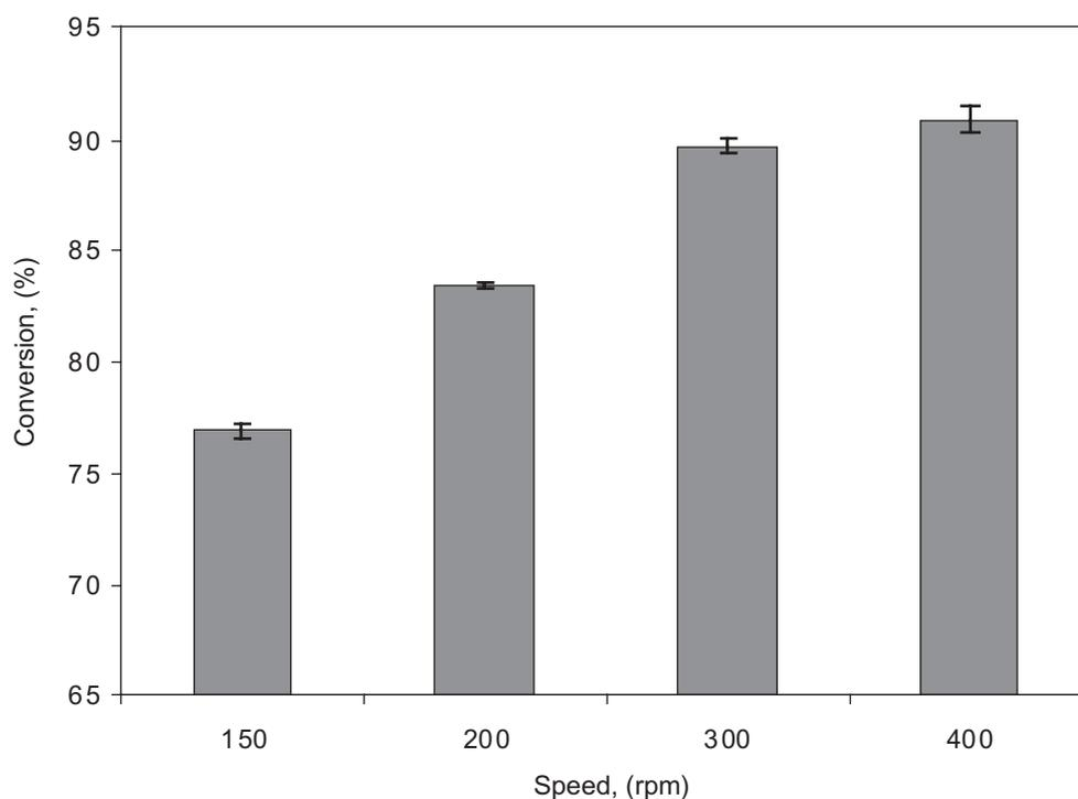
Figure 3. Effect of agitation speed on the esterification of DHSA and 1-octanol. Reaction conditions: reaction time, 3 hr; temperature, 50°C, enzyme concentration, 15% (w/w).
