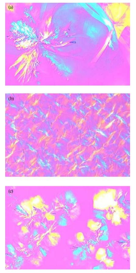
*Figure 2. Polarized light micrographs of (a) palm oil methyl esters, (b) S diesel and (c) mixtures of 70% palm oil methyl esters and 30% S petroleum diesel at -10°C to -50°C (20X magnification).*
