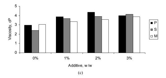
*Figure 5. Effect on (a) pour point, (b) cloud point, and (c) viscosity of blend of mixtures of 80% palm oil methyl ester and 20% petroleum diesel (P, S, and M) in the presence of different concentrations of palm-based additive.*
