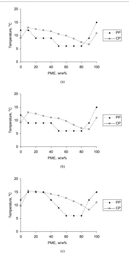
*Figure 1. Cloud point and pour point of palm oil methyl ester (PME) with different petroleum diesels. (a) Diesel P, (b) diesel S and (c) diesel M.*
