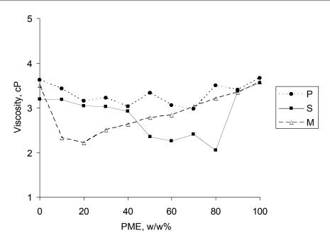
Figure 3. Viscosity of blended palm oil methyl ester (PME) with different petroleum diesels (P, S, and M) at 40°C.
