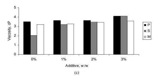
*Figure 4. Effect on (a) pour point, (b) cloud point, and (c) viscosity of blend of mixtures of 70% palm oil methyl ester and 30% petroleum diesel (P, S, and M) in the presence of different concentrations of additive.*
