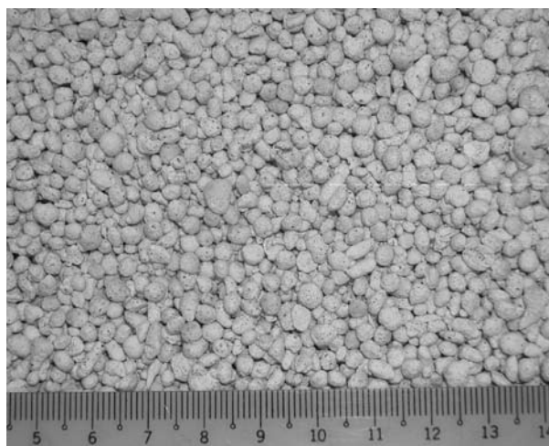
Figure 1. The alginate granule formulation of M. anisopliae containing rice bran as a base nutrient source and kaolin as an inert material.
