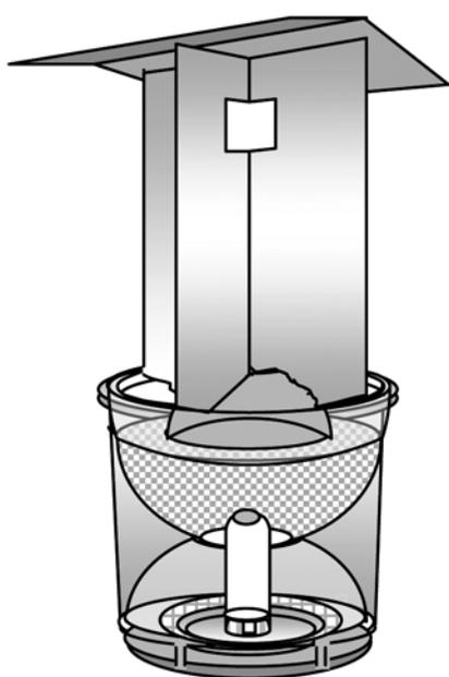
Figure 1. Perspective view of the trap for auto dissemination of spores of *M. anisopliae* into the field.
