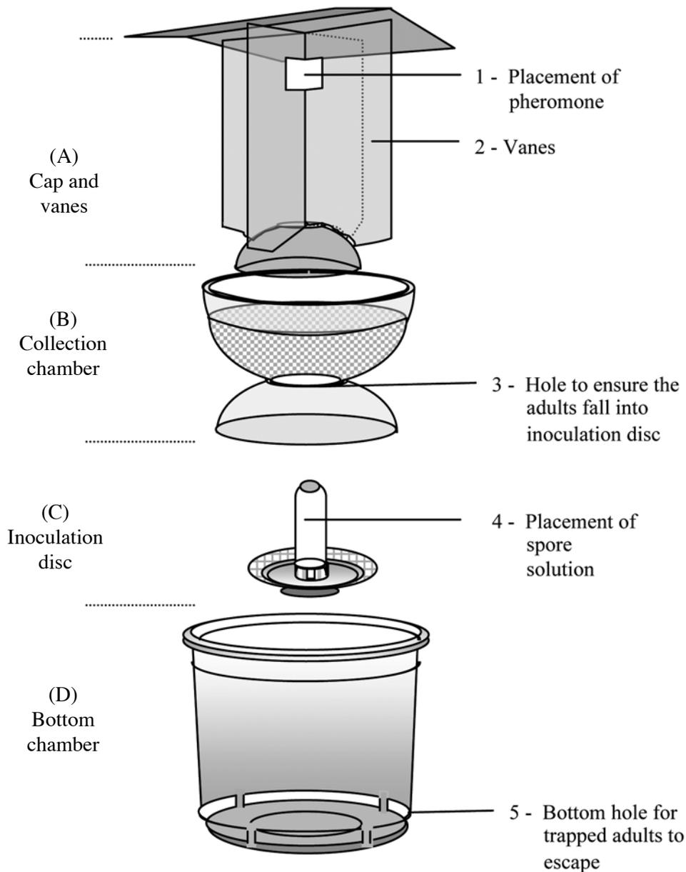
Figure 2. Perspective view of the inoculation trap showing each compartment (A-D).
