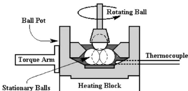
Figure 1. Schematic diagram of four ball wear geometry.
