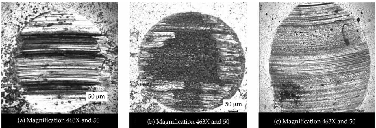
Figure 12. Optical micrographs of wear area on the balls surface and in 600 N (magnification 463X and 50  $\mu\text{m}$ ): (a) palm fatty acid distillate (PFAD) oil, (b) engine mineral oil, and (c) hydraulic mineral oil.
