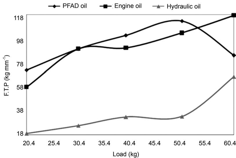
Figure 4. Flash temperature parameter on ball bearings lubricated with palm fatty acid distillate (PFAD), engine and hydraulic oils under different loads.
