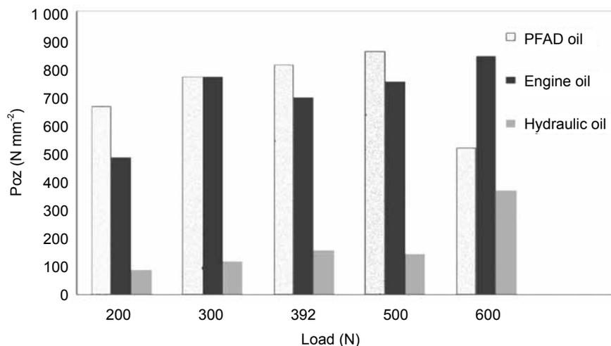
Figure 5. Value of limiting pressure of seizure for palm fatty acid distillate (PFAD), engine and hydraulic oils in 200, 300, 392, 500 and 600 N.
