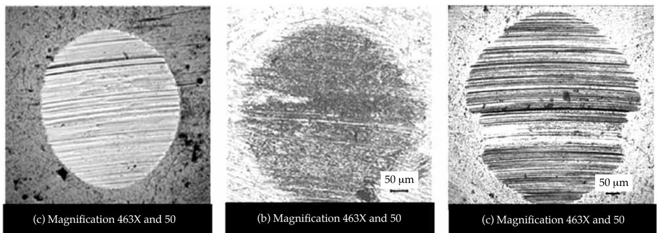
*Figure 9. Optical micrographs of wear area on the balls surface and in 300 N (magnification 463X and 50 µm): (a) palm fatty acid distillate (PFAD) oil, (b) engine mineral oil, and (c) hydraulic mineral oil.*
