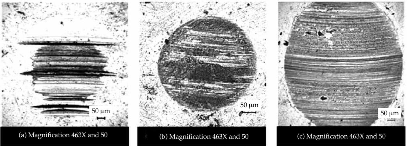
Figure 11. Optical micrographs of wear area on the balls surface and in 500 N (magnification 463X and 50  $\mu\text{m}$ ): (a) palm fatty acid distillate (PFAD), (b) engine mineral oil, and (c) hydraulic mineral oil.
