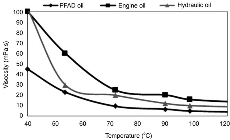
Figure 3. Kinematic viscosity measured for palm fatty acid distillate (PFAD), engine and hydraulic oils under different tested temperature.
