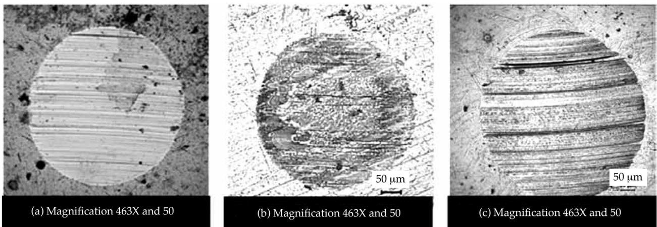
*Figure 8. Optical micrographs of wear area on the balls surface and in 200 N (magnification 463X and 50 µm): (a) palm fatty acid distillate (PFAD) oil, (b) engine mineral oil, and (c) hydraulic mineral oil.*
