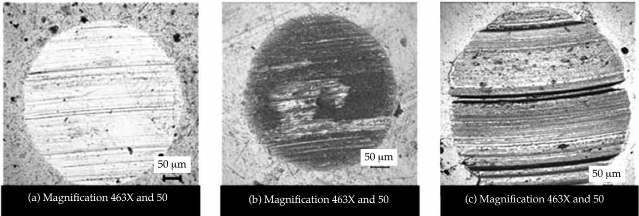
Figure 10. Optical micrographs of wear area on the balls surface and in 392 N (magnification 463X and 50  $\mu\text{m}$ ): (a) palm fatty acid distillate (PFAD) oil, (b) engine mineral oil, and (c) hydraulic mineral oil.
