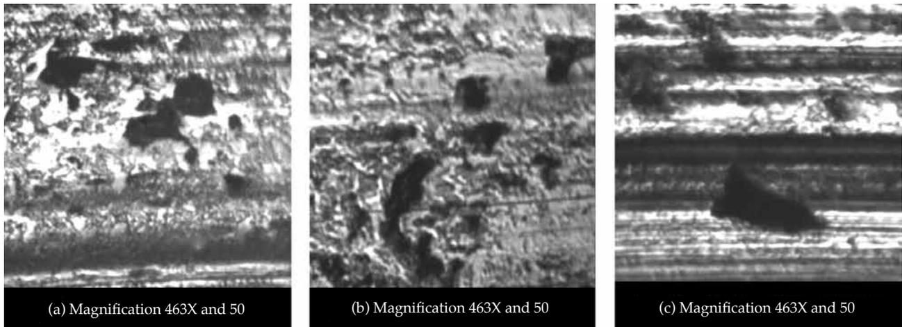
Figure 13. The pitting corrosion on ball specimen. (a) Palm fatty acid distillate (PFAD) ball specimen in 392 N, (b) hydraulic ball specimen in 400 N and (c) hydraulic ball specimen in 600 N.
