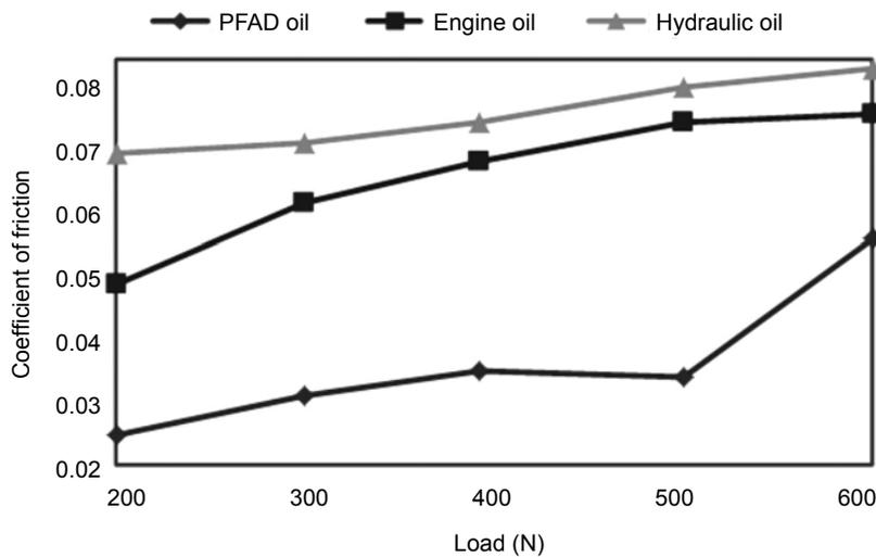
Figure 6. Effect of load on coefficient of friction for palm fatty acid distillate (PFAD), engine and hydraulic oils under 200, 300, 392, 500 and 600 N.
