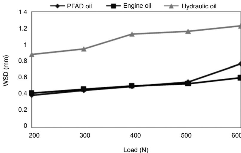
Figure 7. Effect of load on wear scar diameter (WSD) for palm fatty acid distillate (PFAD), engine and hydraulic oils in 200, 300, 392, 500 and 600 N.
