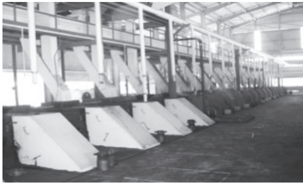
Figure 2. A series of screw presses to crush the palm kernels.
