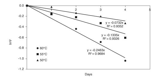
Figure 4. Initial reaction rate of monolaurin yield versus different heat treatment (50°C-60°C) for variables times (1-4 days). Reaction conditions: 8:1 glycerol/lauric acid molar ratio; 1 wt % lipase loading; 200 rpm.
