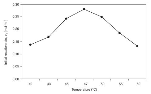
Figure 2. Initial reaction rate of monolaurin yield under different operating temperatures (reaction conditions: 8:1 glycerol/lauric acid molar ratio; 1 wt % lipase loading; 200 rpm)
