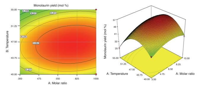
Figure 1. (a) Contour plot (b) response surface plot of monolaurin yield as a function of temperature and substrate molar ratio at fixed lipase loading of 1 wt % lauric acid.
