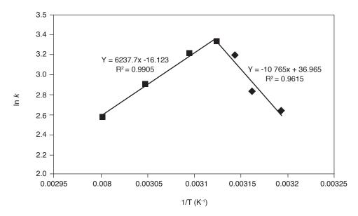
Figure 3. Arrhenius plots for the estimation of activation energy and reversible denaturation energy (40°C-60°C).
