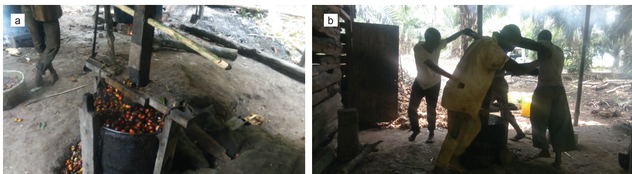
Figure 1. Traditional method of oil extraction used in Buwama-Uganda: (a) manual vertical press with digested oil palm fruits ready for extraction and (b) workers extracting oil manually.
