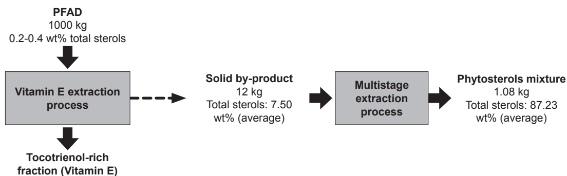
Figure 6. The overall mass balance on the multistage production of phytosterols mixture from palm fatty acid distillate (PFAD).
