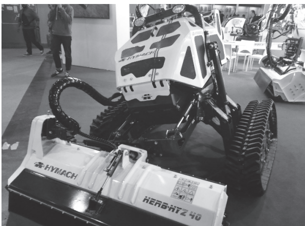
Figure 7. The remote-controlled tool carrier is ideal for slope areas that present the risk of overturning the vehicle with a man on board, or in areas impenetrable by other means.
