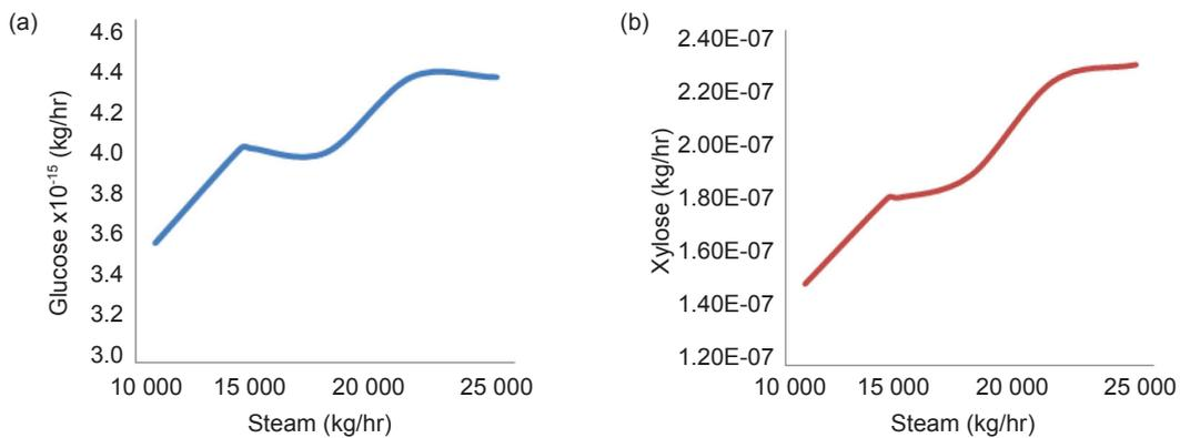
Figure 6. Effect of steam flow rate on production of (a) glucose and (b) xylose in condensate.
