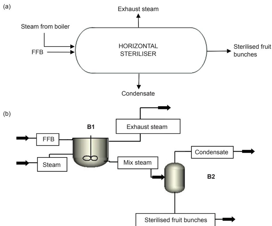
Figure 1. Sterilisation process; (a) schematic diagram and (b) flowsheet diagram in ASPEN Plus.
