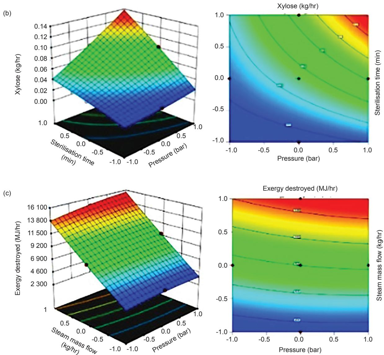
Figure 7. Interactions of (a) sterilisation time against pressure on glucose production, (b) sterilisation time against pressure on xylose production and (c) steam mass flow against pressure on exergy destroyed
