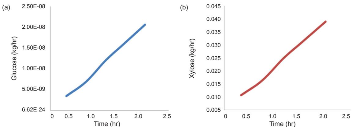
Figure 4. Effect of sterilisation time on production of (a) glucose and (b) xylose in sterilised fruit bunches.
