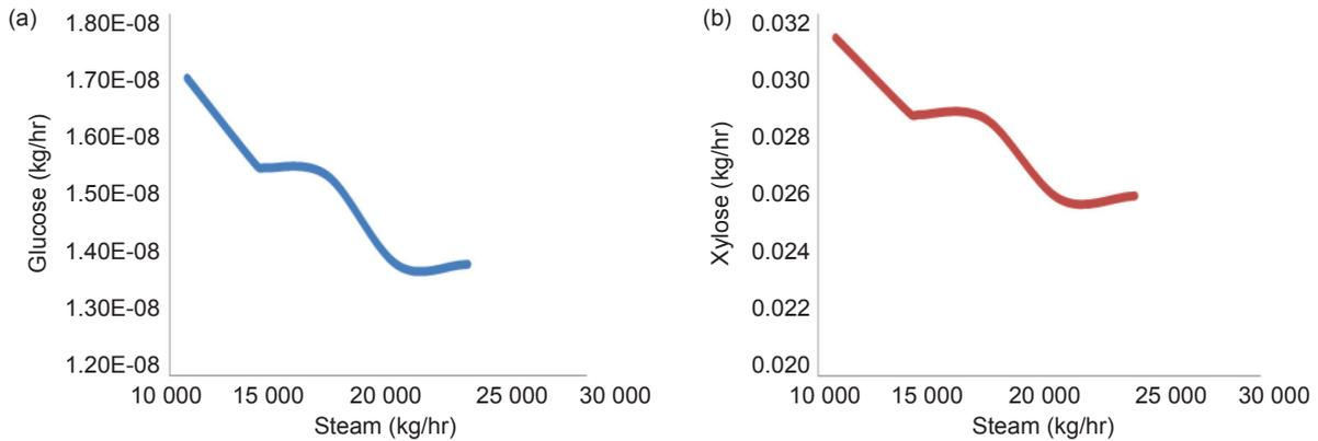
Figure 5. Effect of steam flow rate on production of (a) glucose and (b) xylose in sterilised fruit bunches.
