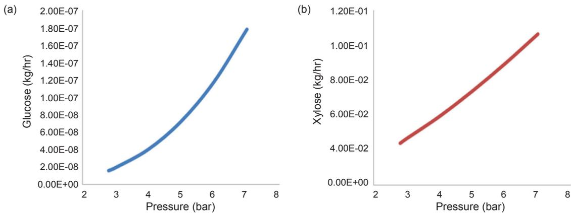
Figure 3. Effect of pressure on production of (a) glucose and (b) xylose in sterilised fruit bunches.
