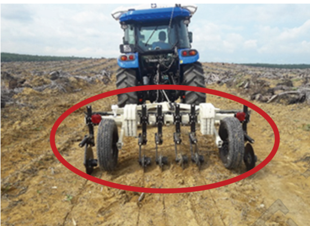
Figure 2. Autopilot tractor-mounted real-time soil EC sensor.
