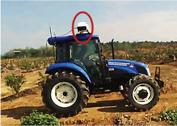
Figure 1. Autopilot tractor-mounted real-time plant N sensor.
