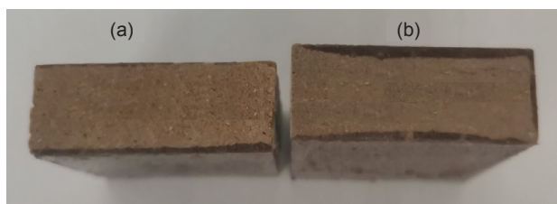
Figure 3. Thickness swelling of MDF 2.0-10 bonded with palm oil-based PU as representation (a) before and (b) after immersed in water for 24 hr.
