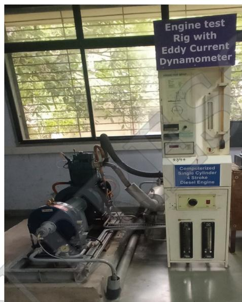
Figure 6. Experimental setup of the engine test rig.
