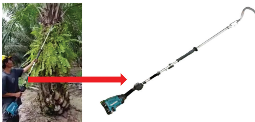
Figure 1. Cantas, a motorised oil palm tree harvester.
