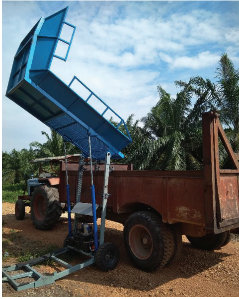
Figure 2. Prototype in tipping position during a field test.
