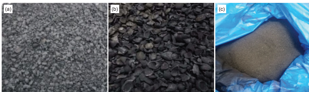
Figure 1. (a) Palm kernel shell biochar (PKSB), (b) activated palm kernel shell (APKS) and (c) fine PKSB and APKS powder after pulverised.
