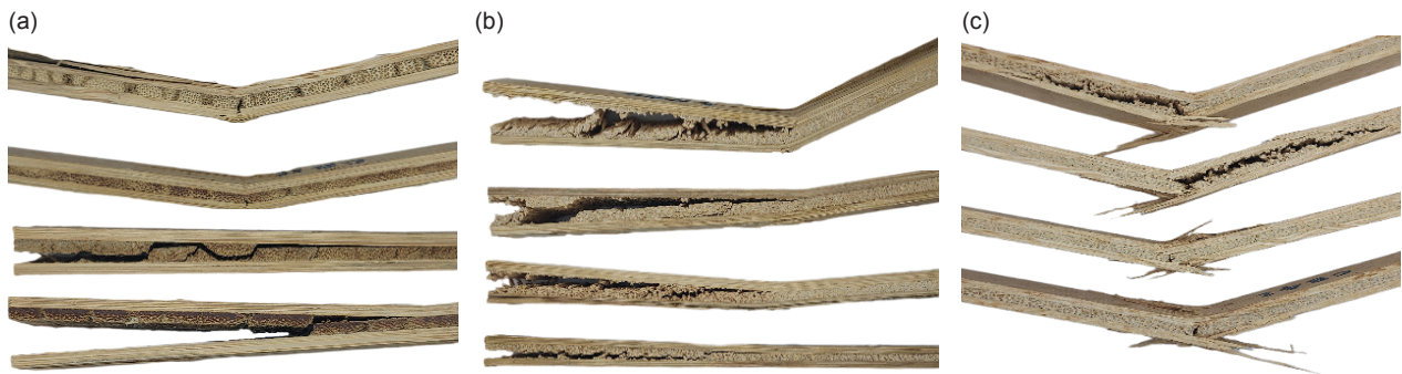
Figure 7. The failure mode of the test specimens after the bending test. (a) Bamboo mats panels, (b) hybrid panels and (c) OPT veneer panels.
